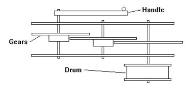
I obtained gears from a cheap toy and rearranged them between two aluminium plates to optimise ratios. The drum was turned from aluminium, the diameter of which obviously depends on your gear ratios and pitch requirements. The formula for the circumference of a circle is "Diameter x 22/7". Additional drums can be turned for different pitch sizes or the number of turns of the 'handle' varied.
