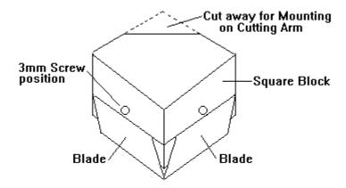
The blades are epoxied to the blocks, and a right angled aluminium plate (or washers) bolted to the outside to keep them in place. It is important for the tips of the blades to meet exactly; the epoxy gives you time to position them accurately and prevent them from moving later under pressure.
